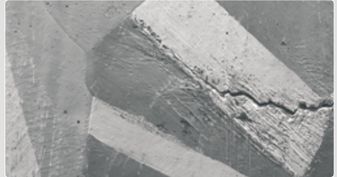
Rissöffnung an Cu-Folie, Oberflächenpräparation mittels FIB (Focused Ion Beam) Crack opening at Cu-film, surface preparation by FIB (Focused Ion Beam)
