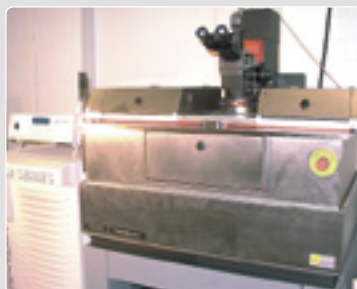
Suss PA 300 –Semiautomatic Wafer Prober (300 mm, shielded)
