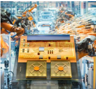
24 GHz transponder module for the wireless localization of tools in production lines (copyright Fraunhofer IZM / Volker Mai)
