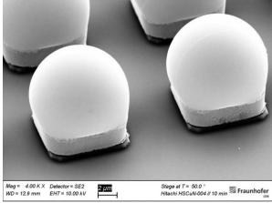
The compact interconnection technology of tomorrow's computers, courtesy of fine pitch contacts made from indium and superconducting metallization.
