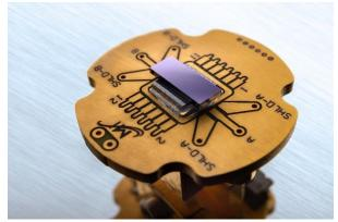
Chip assembly for readout electronics in quantum computers.
