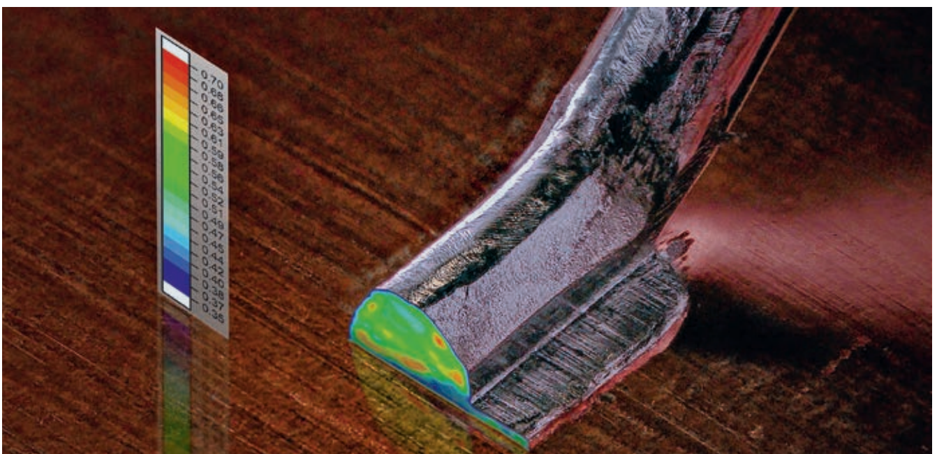
Simulation of shear tests of innovative, aluminum-based thick-wire connections
