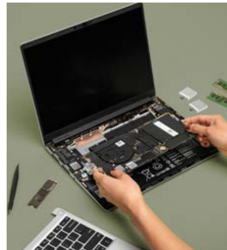
A modular laptop made by Framework with a lifecycle assessment produced by Fraunhofer IZM
