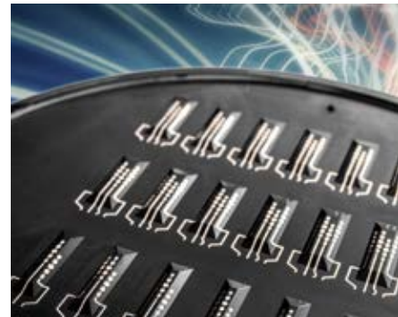
Compression-molded 3D radar antennas in a MIMO array can cover 180° of the surrounding space
