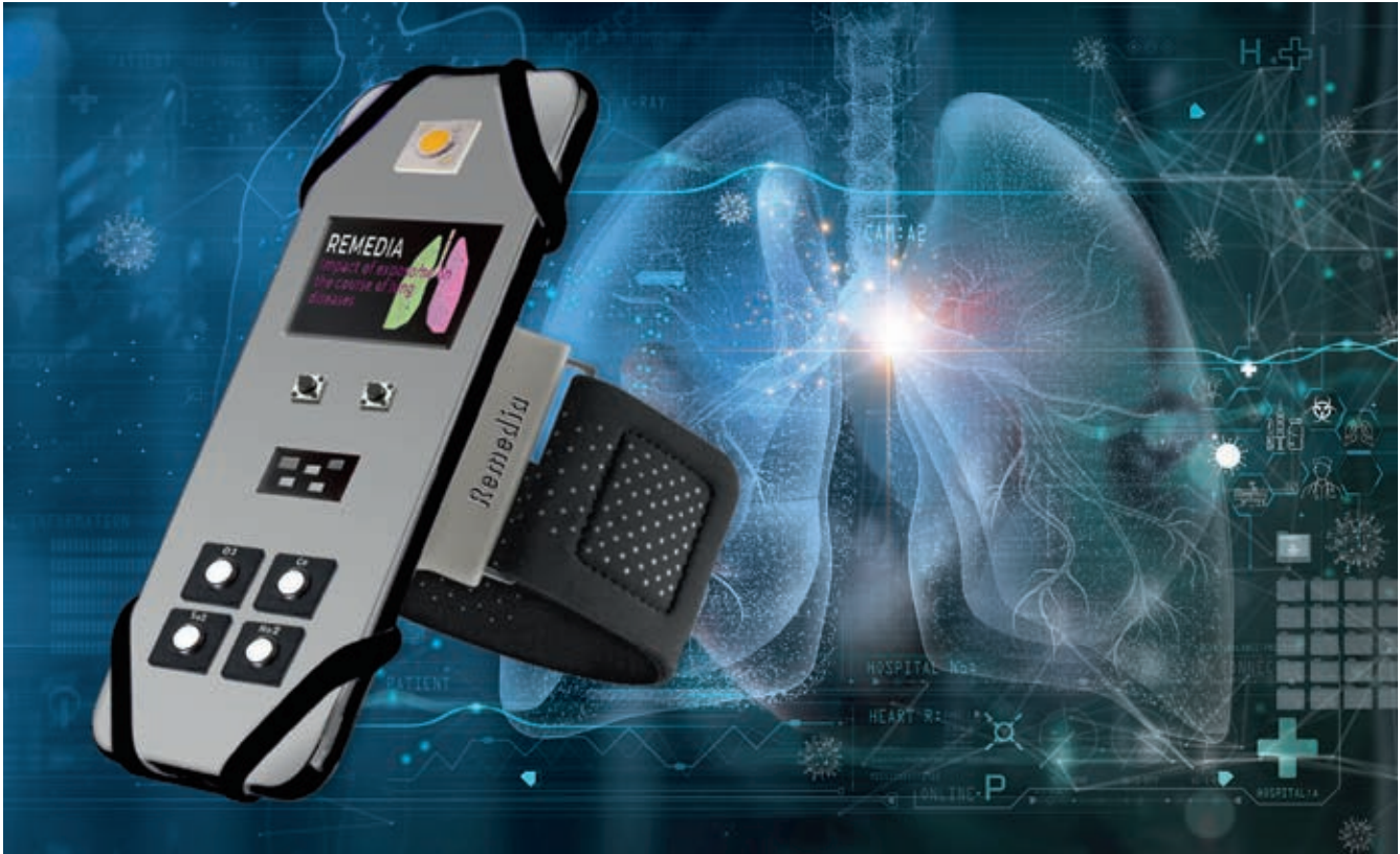
The REMEDIA sensor bracelet keeps track of 40 environment factors to see which affect respiratory diseases
